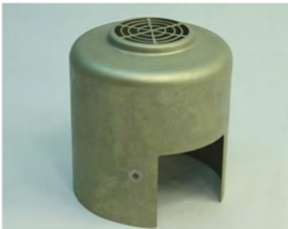
6061 Aluminum, chromate conversion anodize finish. Custom cover for a military motor. 5.00" diameter X 6.50" height x 0.040" thick aluminum formed using hydroforming.
