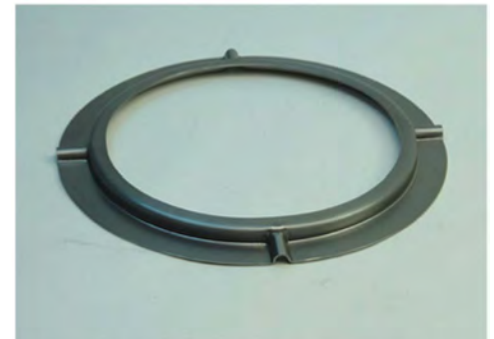
16ga 1008 steel formed using hydroforming, 9.25" diameter X 0.375" height.
