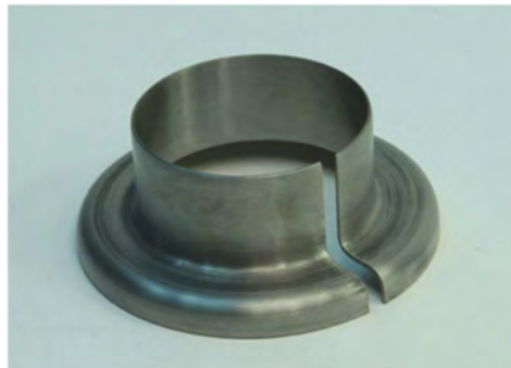
16 gauge 304 s/s, 3.00" od. X 1.50" height, formed using hydroforming.
