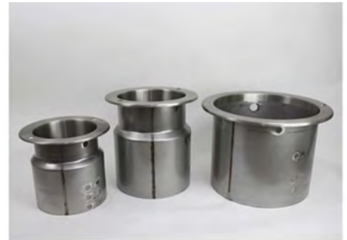
13 gage 304 s/s inner housings for high pressure cookers. Diameters are 12" to 24" and height is 18". Formed using automatic seam welded cylinder and metal spinning.
