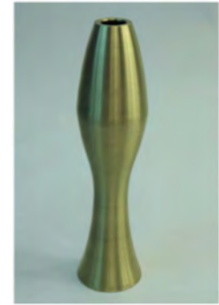
Brass Door handle used on a commercial building in Manhattan, NY. Customer needed the part to be completely hollowed and light weight in order to prevent handle from shattering the 10 foot glass doors. Helander Metal Spinning had the solution. 12" height X 3" diameter X 0.060" Brass, produced 350pcs for one building.
