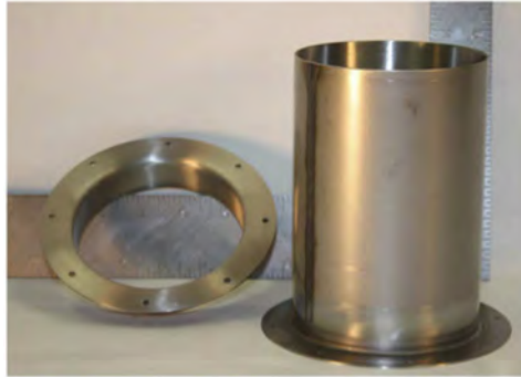
Air filtration sleeves and rings, 16 gage 304 s/s, ID polished to a #4 finish. 6" diameter od to 7" long.
