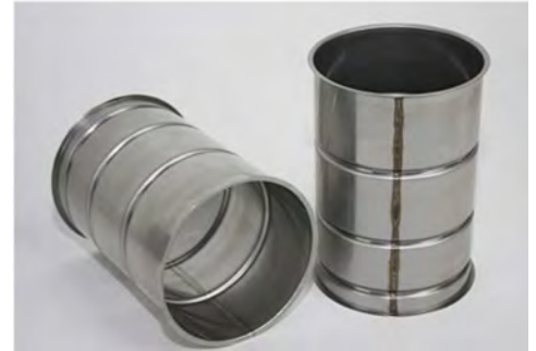
Air filtration cartridge, 26 gage 304 s/s 6.25" height X 4" i.d. Made via CNC spinning and cylinder/tube welding.
