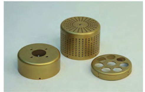
Gold Anodized 0.040" Aluminum, electrical housing, three piece assembly. 3.00" diameter X 4.00" height.
