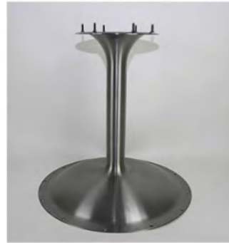
Heavy duty table column end table column, three piece welded construction polished seamless with welded studs. 25" diameter X 39" height x .075" thick steel.
