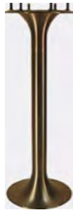
End table column, three piece welded construction polished seamless with welded studs. 9" od. X 24" height X .075" thick steel.
