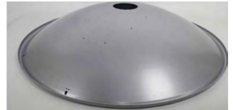
High Precision 42" diameter X 8" height 6061-0 aluminum 0.080" thick .020" RMS. Clear anodized.
