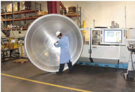
2011 photo on an 8 foot satellite dish spun at Helander. 99.38" diameter X 15.50" tall, 0.125" aluminum. +/- .060" gap on tolerance.
