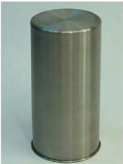
304 s/s 6.80" height 3.4" diameter x 0.040" thick used to house +/- .005" tolerance plutonium bars. Formed via hydroforming and spinning.
