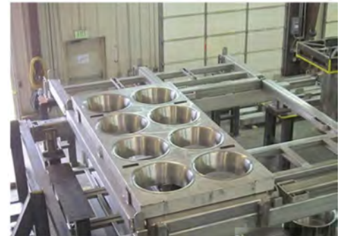
Customer picture of assembly for waste storage project using flanged cones spun at Helander Metal Spinning Company.
